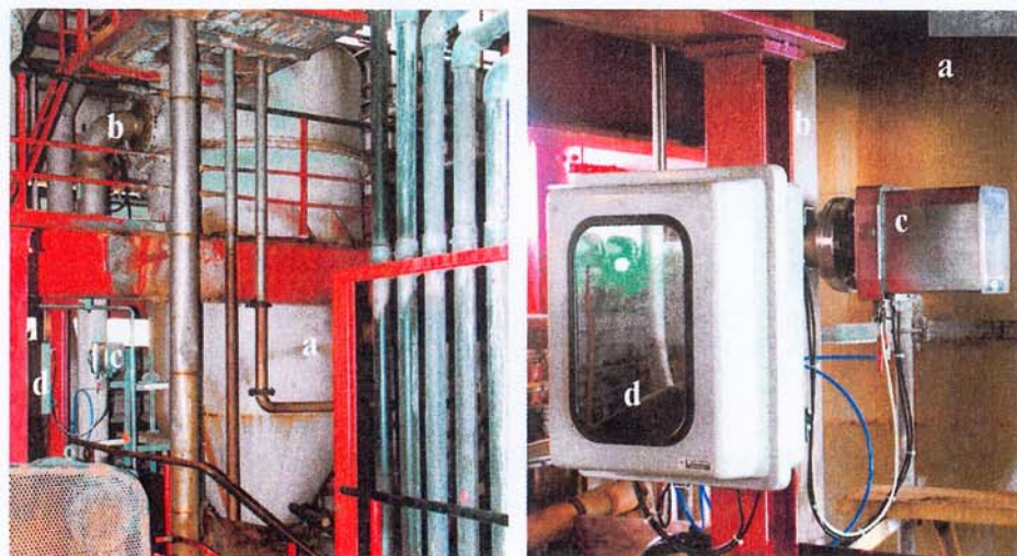
Fig. 4: Opus installation: a) crystalliser, b) recirculation loop, c) Opus, d) control box
