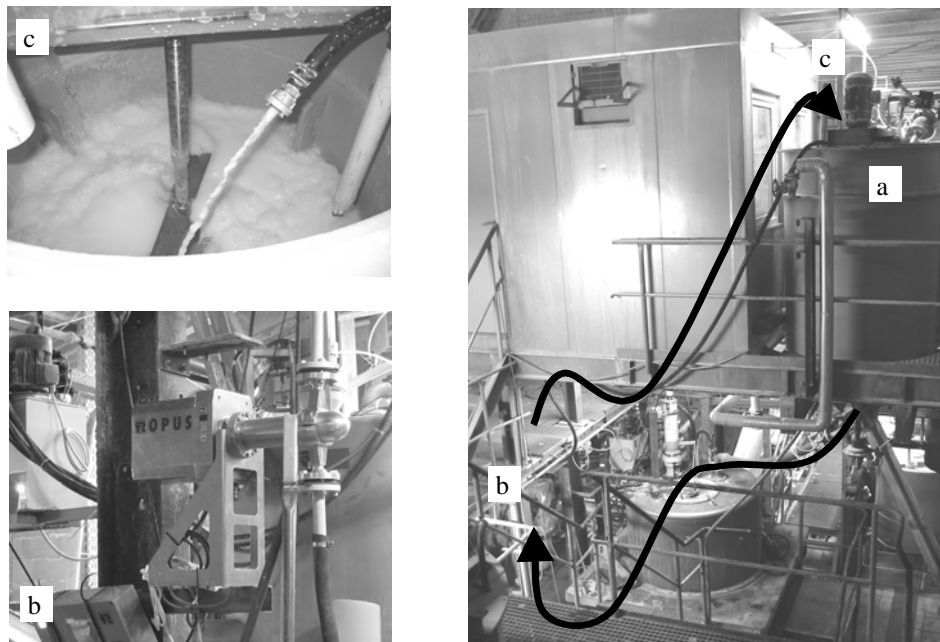
Fig. 5: OPUS installation in industrial environment. a) Crystallizer (1700 l), b) OPUS, c) Re-circulation flow
