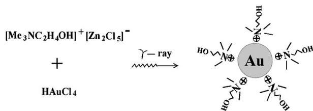
**Scheme 1.** Stabilized gold nanoparticles formed in RTILs under  $\gamma$ -irradiation.
