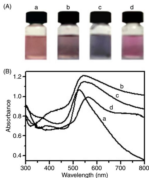
**Figure 4.** (A) Photographs of the gold nanoparticles obtained from the solutions of (a) sample 1, (b) sample 2, (c) sample 3 and (d) sample 4. (B) UV–vis absorption spectra corresponding to (a)–(d) in photographs.
