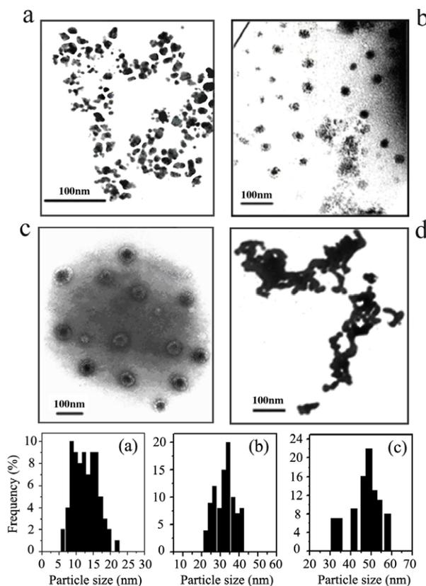
**Figure 1.** TEM images of gold nanoparticles formed in (a) QAIL (sample 1); (b) QAIL + 2-PrOH (sample 2); (c) QAIL + H<sub>2</sub>O (sample 3); (d) H<sub>2</sub>O (sample 4).
