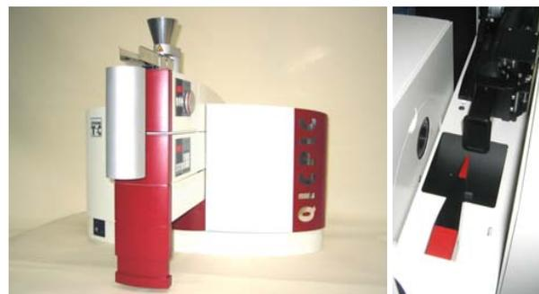
Figure 2: (a) DIA sensor QICPIC with dry disperser RODOS/L inserted in the measuring zone, (b) view of the outlet of the dispersing line and vacuum inlet in the measuring zone.
