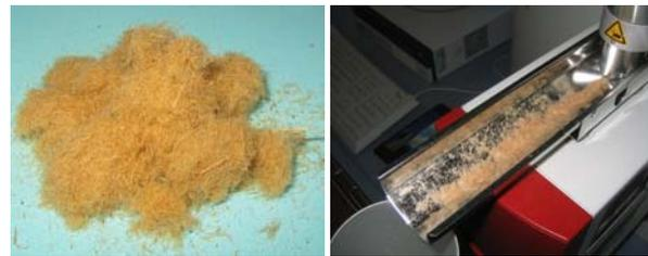
Figure 5: Wood fibres are manually pre-dispersed in the V-chute of a vibratory feeder dosing the fibres into the dry disperser RODOS/L for DIA.
