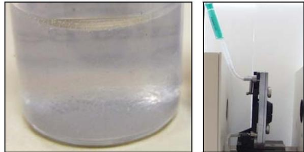
Figure 9: (a) highly transparent gel particles of about 1 mm diameter suspended in water, (b) pumped by a syringe through a flow cell with 2 mm optical path length.
