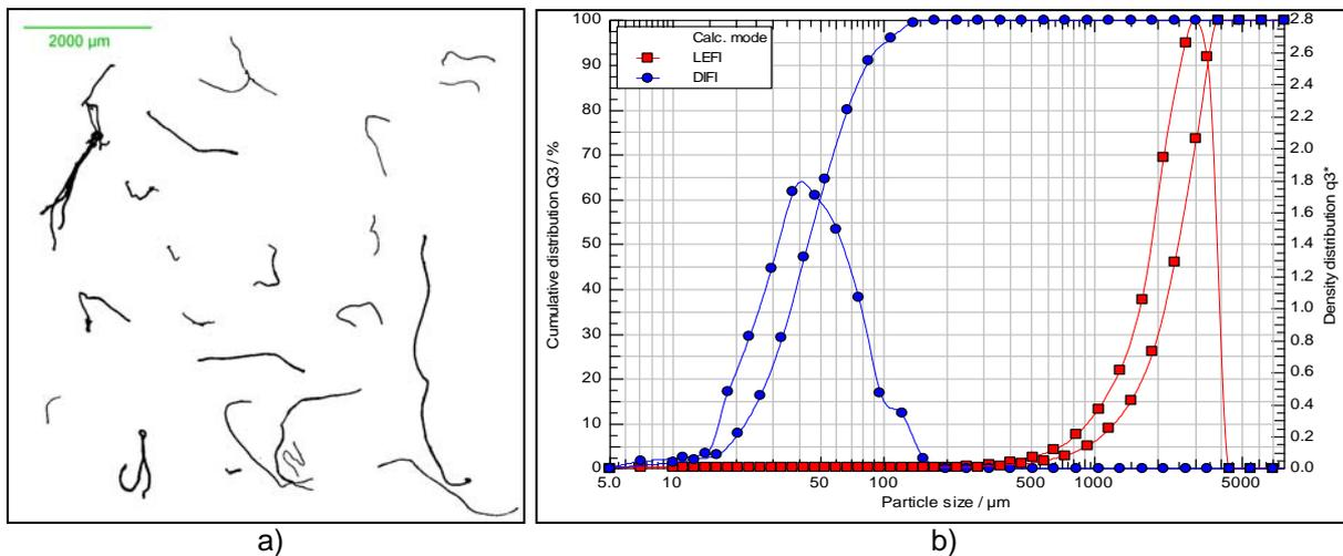
Figure 4: The distributions of length and diameter and a sample image of recycling fibres, measured by QICPIC, with the measuring range R7 (10 µm to 3410 µm) and the dry disperser RODOS/L with injector diameter 4mm.
