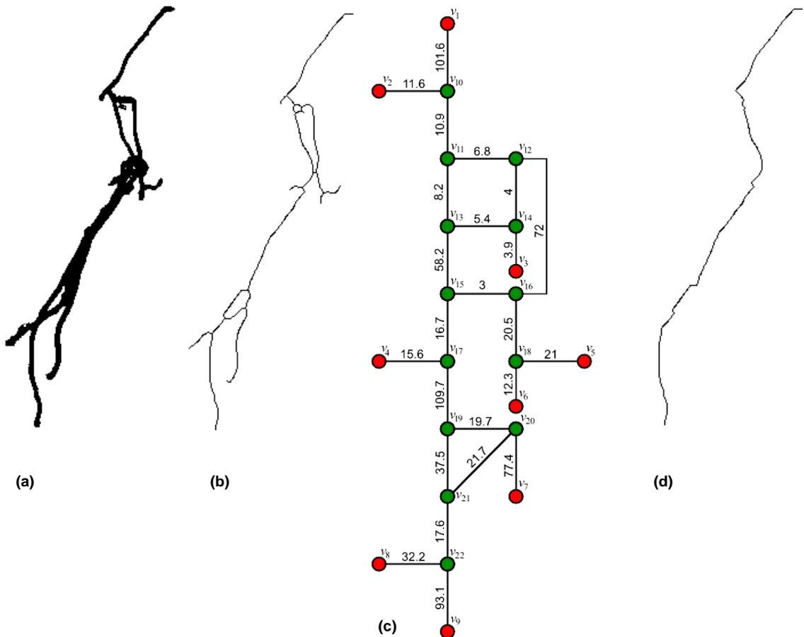
Figure 2 (a)-(d): Skeletonization and graph transformation of a fibre particle
